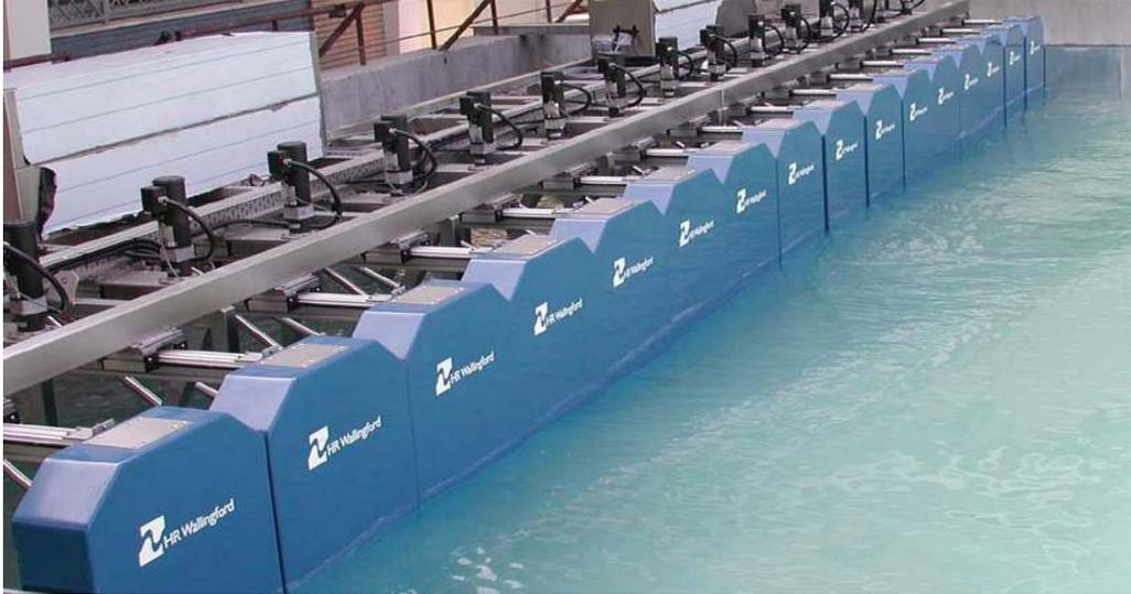
Fig 6.2: UTP basin wave maker system
