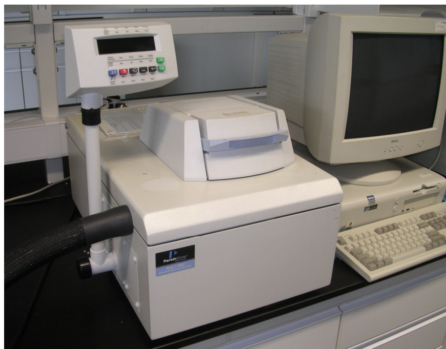
Figure 4.5-3 Thermogravimetry (TG) Analyzer
