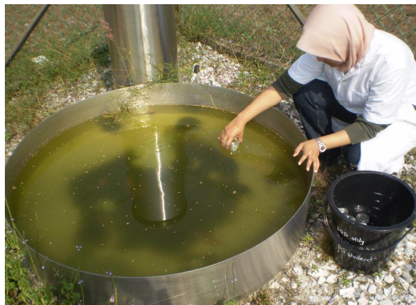
Figure 3.3 Sampling of water from evaporation pan, meteorological station, UTP
