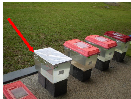
Figure 3.13 Aluminum foil was used for sealing purpose
