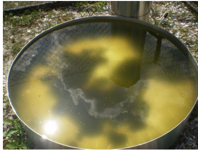
Figure 3.4 Algae as indicated by yellowish green color of the water in evaporation pan
