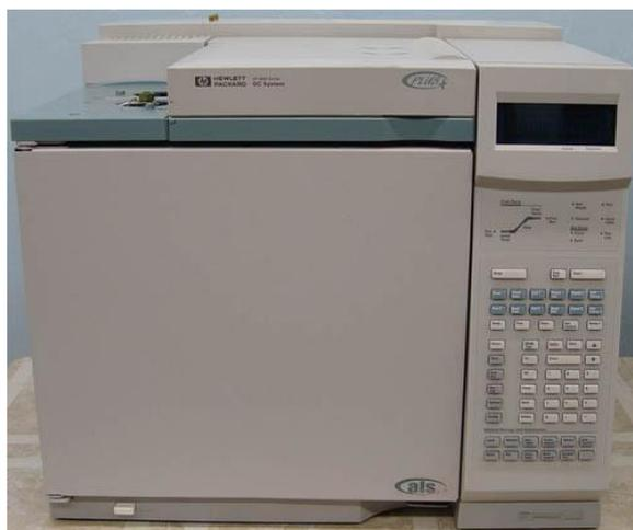
Figure 3.7: The GC 6890 series by Hewlett Packard
