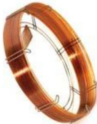
Figure 3.8: Image of a Gas chromatograph column [112].
