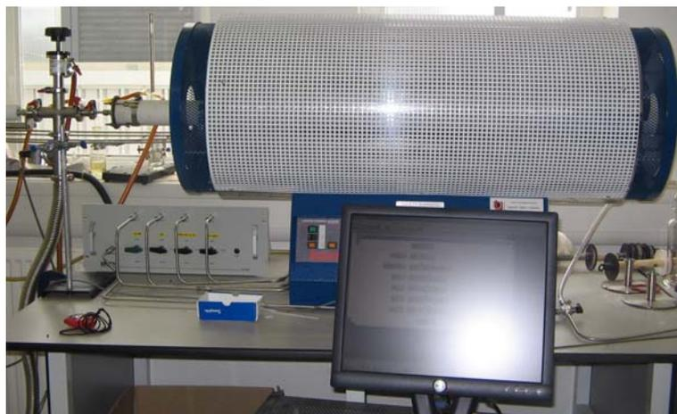
Figure 4.2 Preliminary experimental setup of thermal CVD
