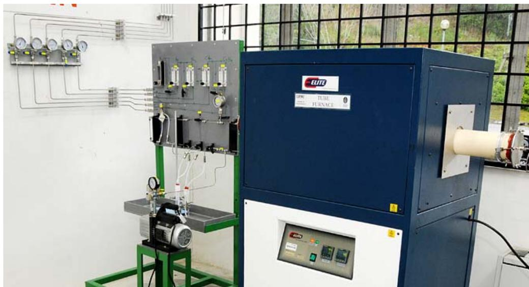
Figure 4.4 Modified experimental setup of the modified thermal CVD
