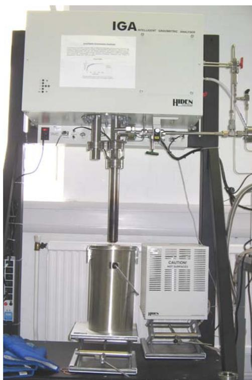
Figure 4.7 Intelligent gravimetric analyzer
