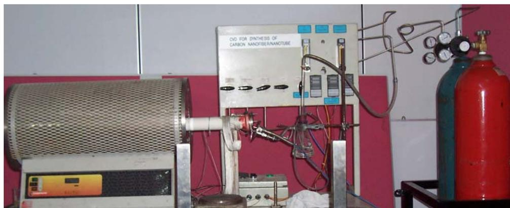
Figure 4.6 Experimental set up of FC-CVD system in the lab
