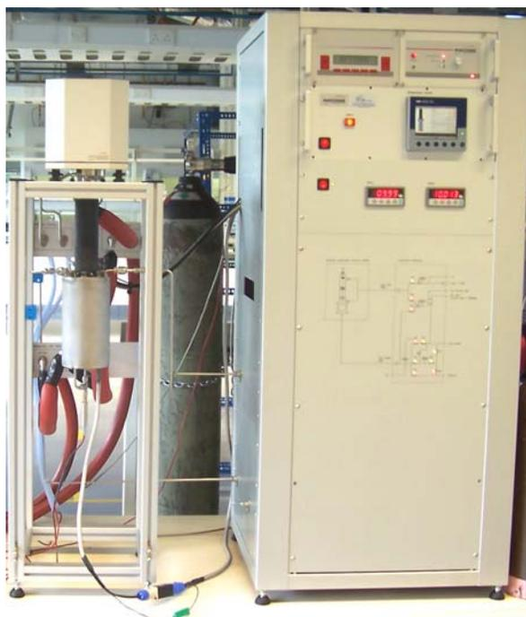
Figure 4.8 Magnetic suspension balance
