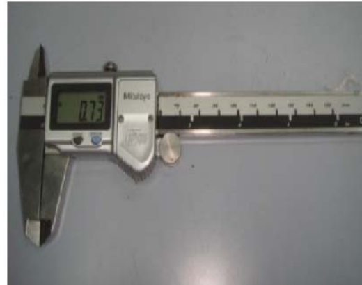
Absolute Coolant Proof Caliper (No.99MAD011B) Resolution= 0.01mm Repeatability= 0.01mm Accuracy= +/- 0.02mm Operating Temperature=0 to 40 °C Made in Japan
