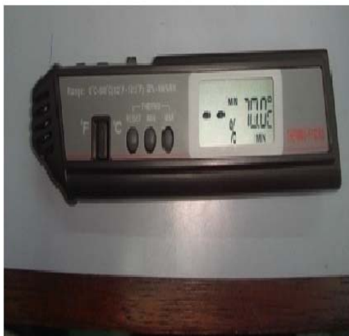
Thermo-Hygrometer Temperature Range= 0 °C - 50 °C , 32 °F - 122 °F Resolution= 0.1 °C Accuracy= +/- 1 °C Humidity Range (2%-98%) RH Resolution= 1 %RH Accuracy= +/- 5 %RH
