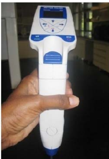
Portable Density Meter (type: Densti30P) Made in Japan (METTLER TOLEDO) Accuracy \pm 0.0005 Temperature range (10-40) ^{\circ}\text{C}
