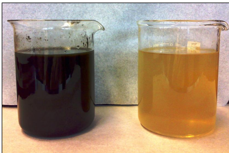
Figure 3.1: Real wastewater before (left) and after (right) pre-treatment
