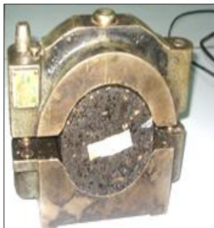
Figure 2-1: Curved steel loading plates used in the Marshall Test set-up
