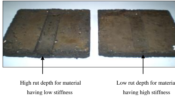
Figure 3-17: Wheel tracking specimen with different rut depth
