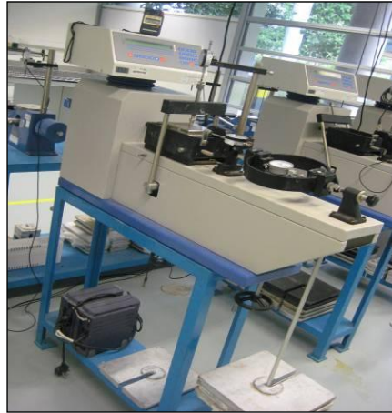
Figure 3-9: Direct shear box apparatus with different load
