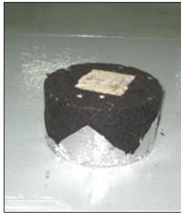
Figure 3-13: Specimen for Creep test
