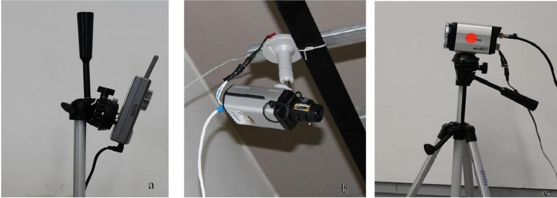
Figure 5.2: Video acquisition devices: a) D'link DCS-2120, b) Samsung SNB-3000 and c) Samsung SDZ-375.
