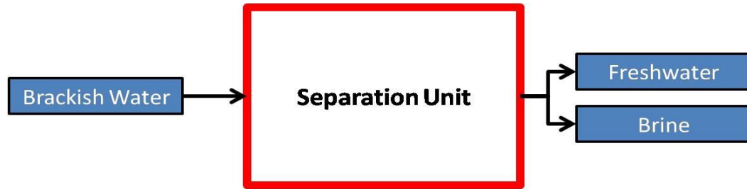
Figure 1.1: Input – Output Diagram of Desalination Process
