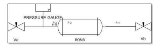
Figure 5: Initial Volume,  $V_i$  ( $V_a$  to  $V_b$ )
