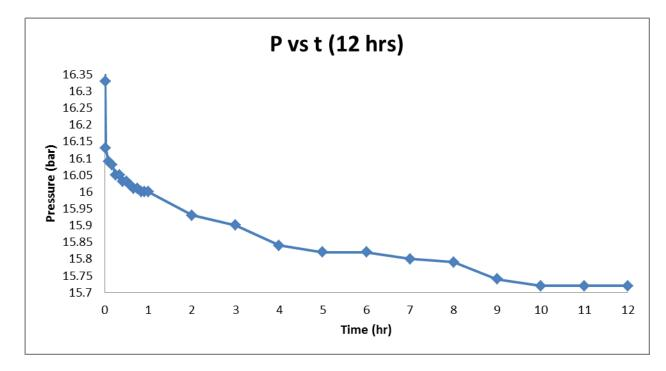
Figure 10: Pressure vs time for DEA at 20 bar (12 hour)
