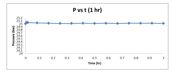
Figure 11: Pressure vs time for DEA at 30 bar (1 hour)
