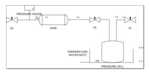
Figure 6: Volume 1,  $V_1$  ( $V_a$  to  $V_c$ )
