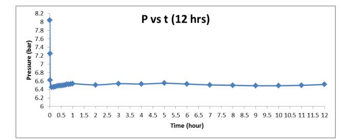
Figure 8: Pressure vs time for DEA at 10 bar (12 hour)
