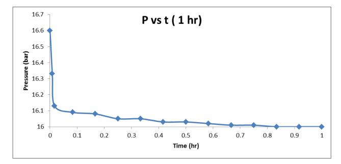
Figure 9: Pressure vs time for DEA at 20 bar (1 hour)
