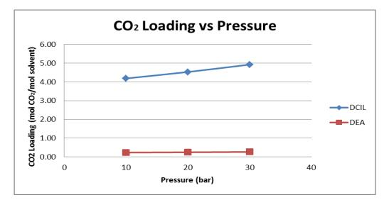
Figure 18: CO<sub>2</sub> loading vs pressure for DEA and [P<sub>888</sub>C<sub>10</sub>P<sub>888</sub>] docusate
