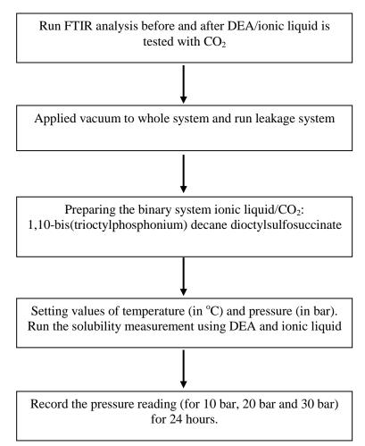
Figure 2: Process flow diagram for methodology
