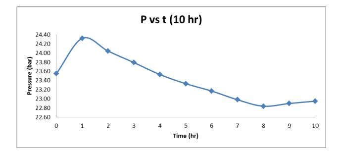
Figure 15: Pressure vs time for  $[P_{888}C_{10}P_{888}]$  docusate at 30 bar (10 hour)
