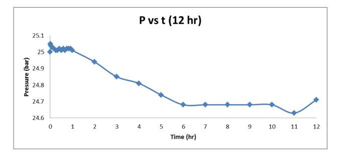
Figure 12: Pressure vs time for DEA at 30 bar (12 hour)
