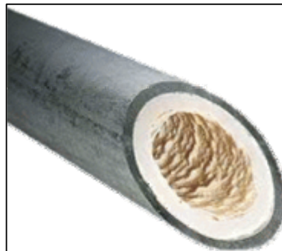
Figure 1 : Scale deposit inside surface pipeline.
