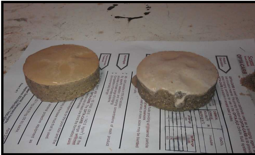
Figure 24: Mud Cake using OPTA CARB
