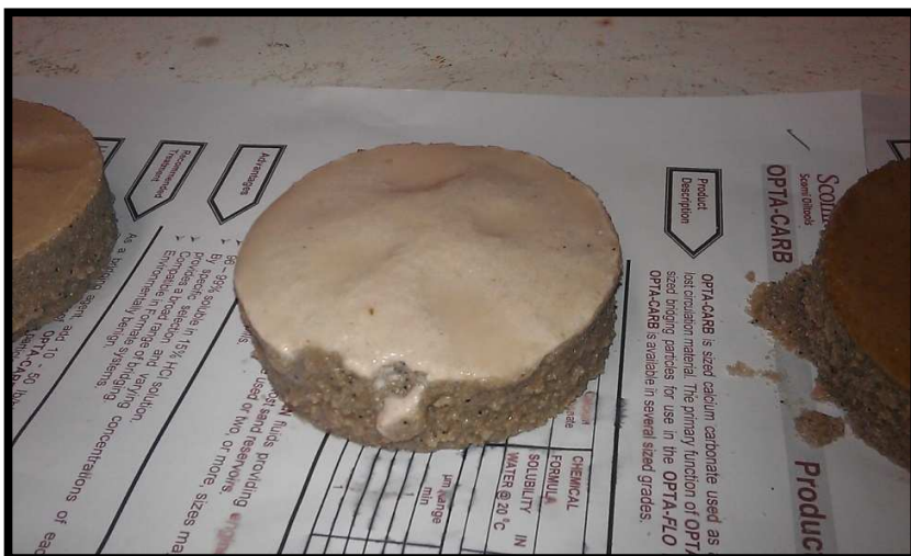
Figure 25: Mud Cake Using OPTA CARB
