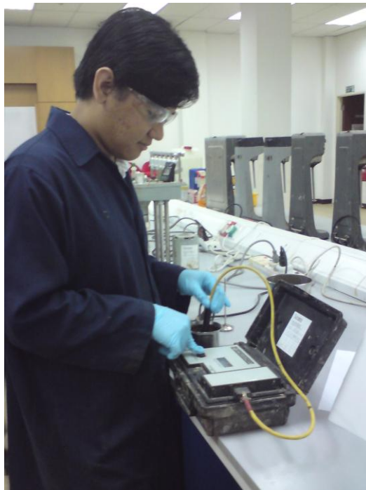
Figure 10: The emulsion stability test using ES meter.
