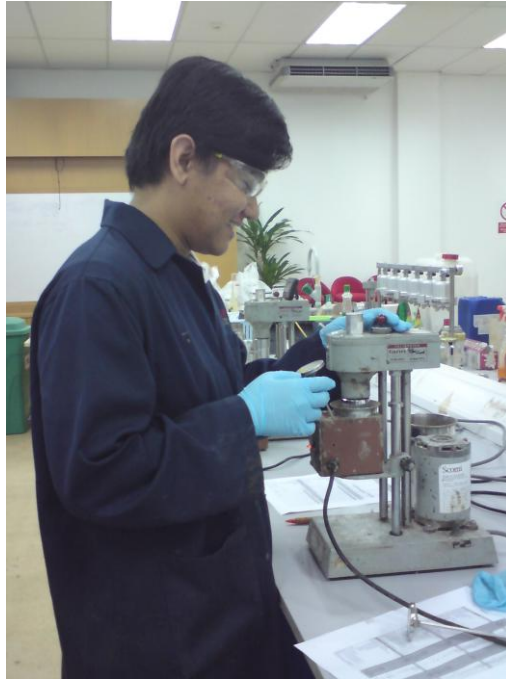
Figure 9: Rheology test using Fann 35 Viscometer.
