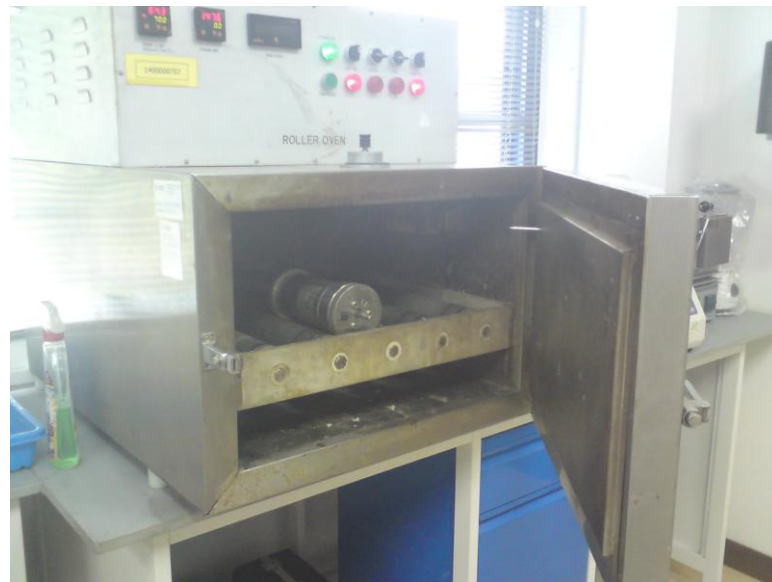
Figure 11: Samples being hot roll in the oven.
