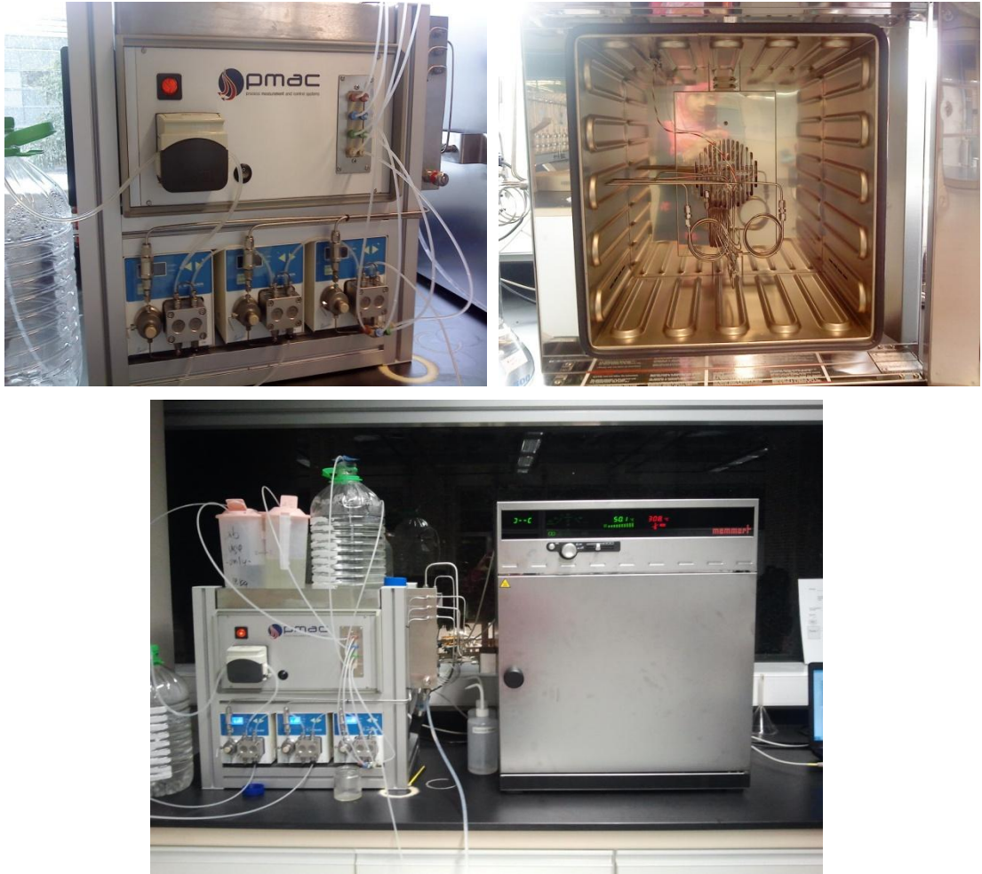
Figure 17: The equipment for dynamic tube blocking testing of scale inhibitors
