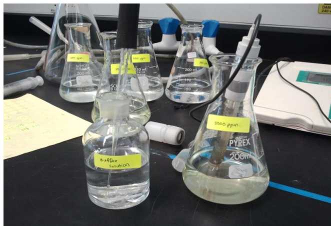
Figure 12: Buffer solution was diluted in SI/SW and measured by pH meter
