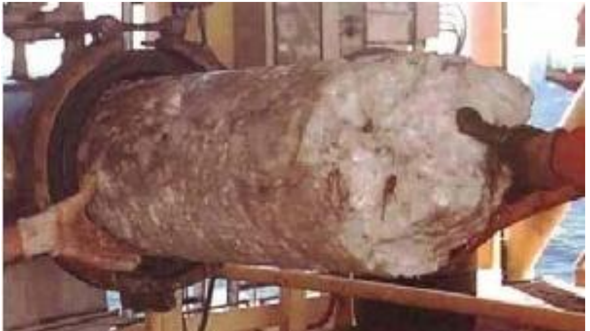
Figure 3 Gas hydrates plug in a pipeline
