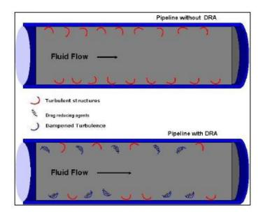
Figure 5: Illustration of dampened turbulence after DRA injection
