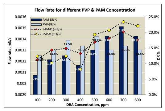
Figure 28: Effect of flow rate of fluid versus PVP and PAM concentrations
