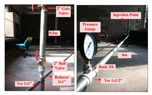
Figure 16: Injection point to first pressure gauge
