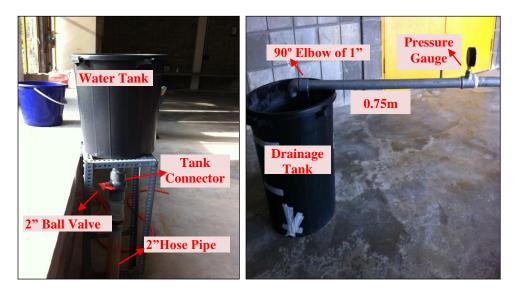
Figure 14: Water tank and drainage tank
