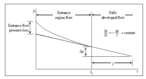
Figure 3: Pressure distribution in horizontal pipe
