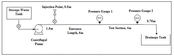
Figure 13: Schematic Diagram of Experiment Setup
