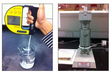
Figure 19: Digital density and Fann Viscometer
