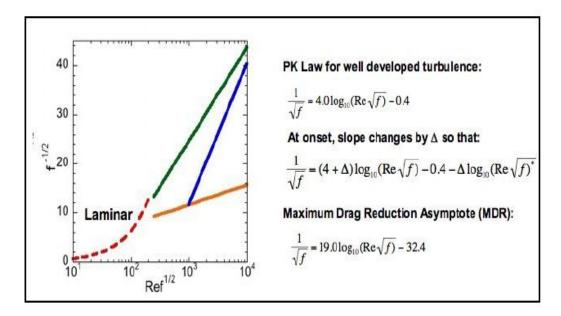
Figure 7: Prandtl-Karman plot for representing polymer drag reduction
