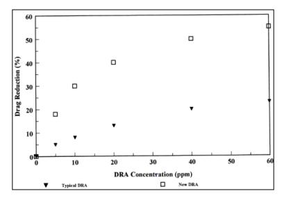
Figure 1: Drag Reduction Performance Single Phase Oil Flow
