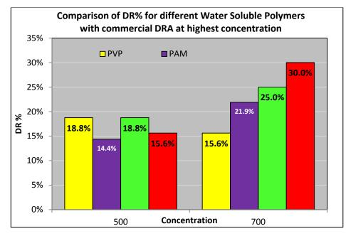
Figure 32: Effect of DR% versus water soluble polymers concentrations with comparison to commercial DRA
