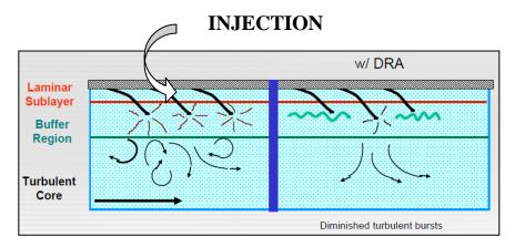
Figure 4 : Drag Reduction Mechanism
