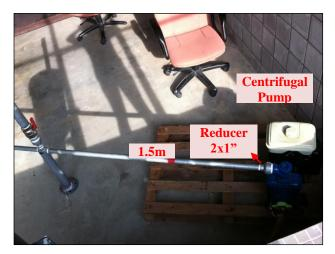
Figure 15: Centrifugal pump to injection point
