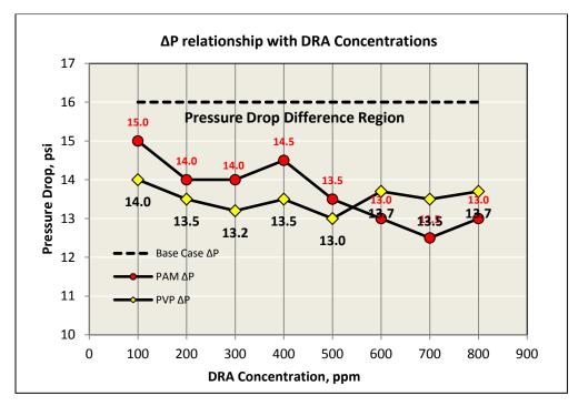
Figure 27: Effect of pressure drop of base case compared with pressure drop of PVP and PAM versus different concentrations
