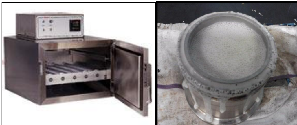
Figure 15: Roller oven (left), Mud sample after aging at high temperature (right)
