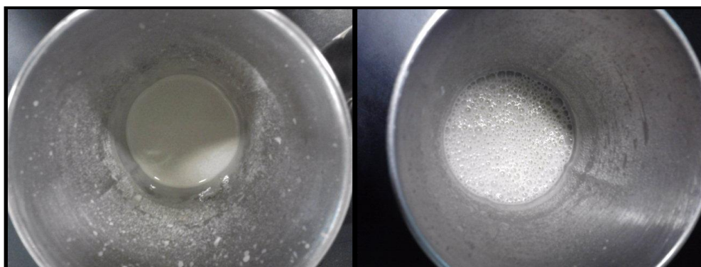
Figure 11: Drilling fluid after mixing – base mud (left), mud with surfactant (right)
