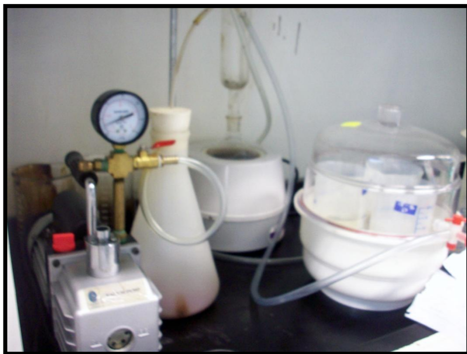
Figure 8: Desiccators with vacuum pump.
