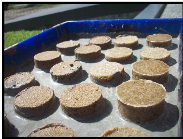
Figure 6: Core sample preparation
