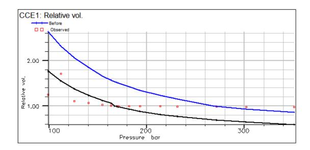
Figure 4.8: Comparison of regression result by tuning of AF using SRK model
