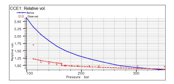
Figure 4.5: Comparison of regression result by tuning of all three variables using SRK model
