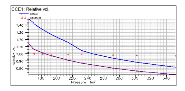
Figure 4.2: Comparison of regression result by tuning of Tc using PR model
