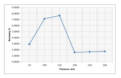
Appendix 11: Pressure vs Recovery Data for PR model of tuning Pc using 500 grid size
