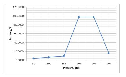
Appendix 15: Pressure vs Recovery Data for SRK model of tuning Pc using 500 grid size
