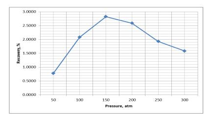
Appendix 12: Pressure vs Recovery Data for PR model of tuning AF using 500 grid size
