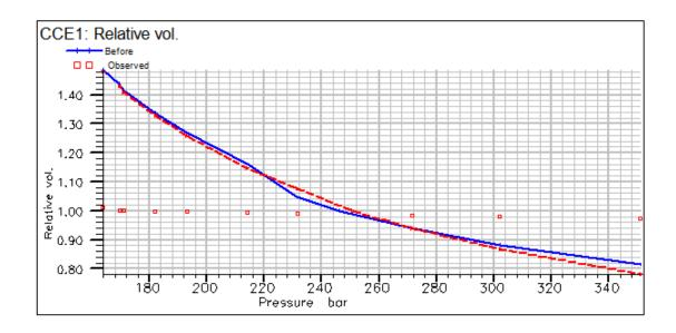
Figure 4.3: Comparison of regression result by tuning of Pc using PR model
