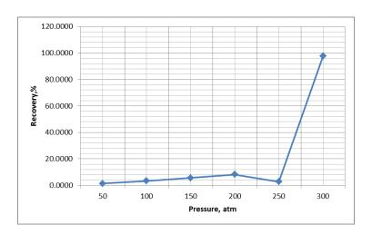
Appendix 16: Pressure vs Recovery Data for SRK model of tuning AF using 500 grid size
