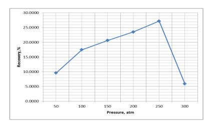
Appendix 14: Pressure vs Recovery Data for SRK model of tuning Tc, using 500 grid size
