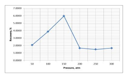
Appendix 13: Pressure vs Recovery Data for SRK model of tuning Tc, Pc & AF using 500 grid size
