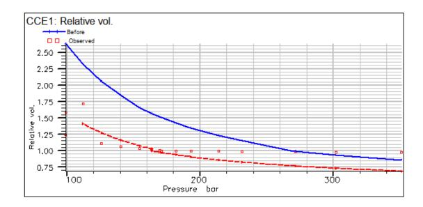
Figure 4.6: Comparison of regression result by tuning of Tc using SRK model
