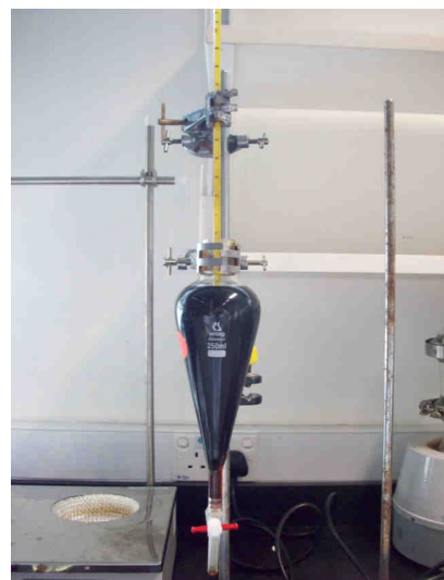
Figure 2.2: Acid extraction experiment during gravity separation
