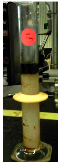
Figure 12.2 Effluent from Water flooding (1% \text{NaCl} )
