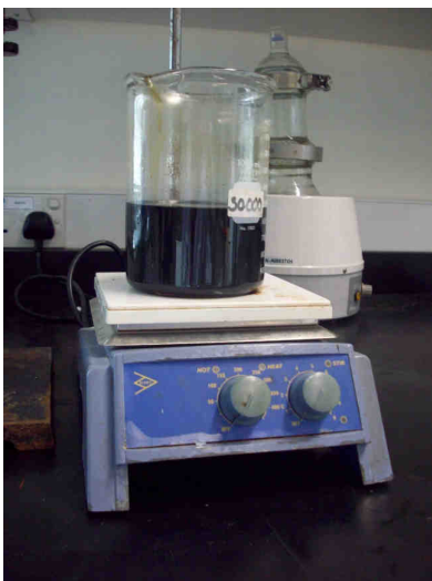
Figure 2.1: Acid extraction experiment during mixing process
