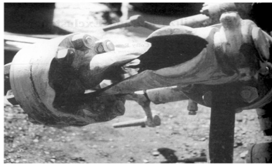
Figure 7 : Surface choke failure due to erosion of formation sand
