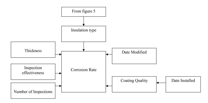
Figure 3.6: Flowchart of External CUI SCC for Austenitic Stainless Steels (cont) [9]
