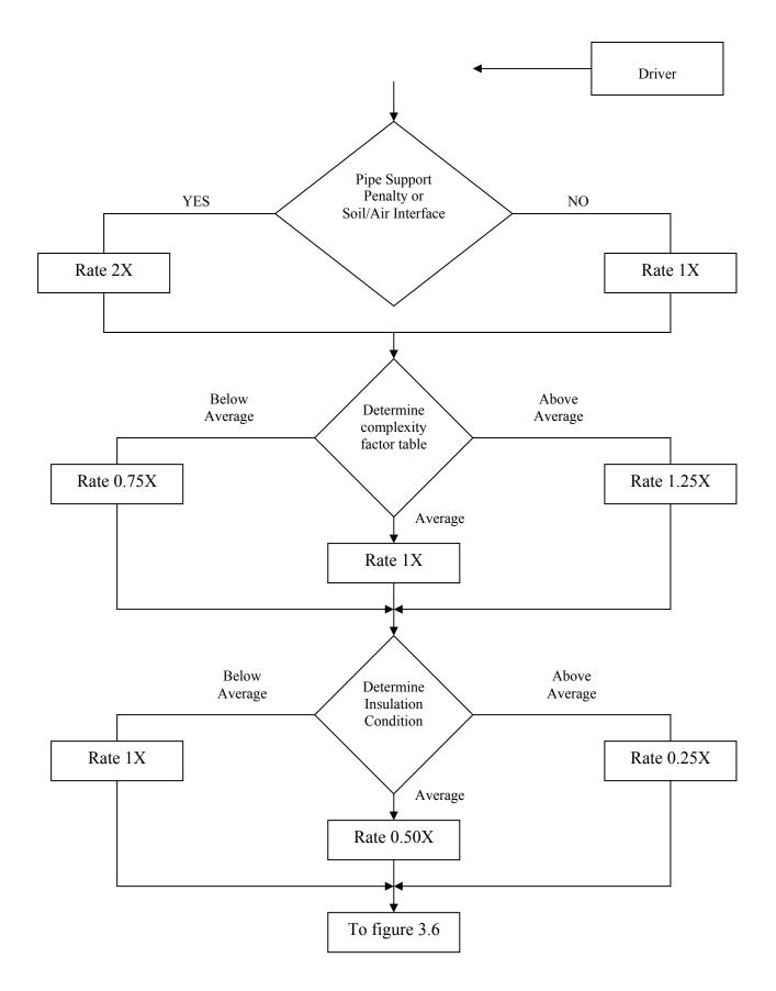
Figure 3.5: Flowchart of External CUI SCC for Austenitic Stainless Steels [9]
