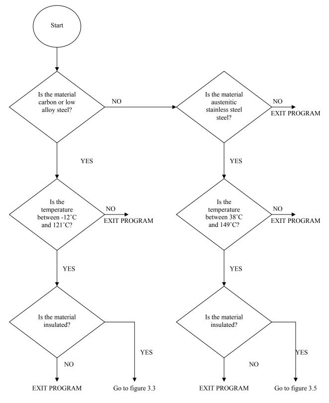
Figure 3.2: Flowchart for External Damage [9]
