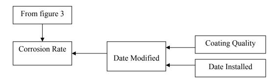
Figure 3.4: Flowchart of CUI for Carbon Steel (Cont) [9]
