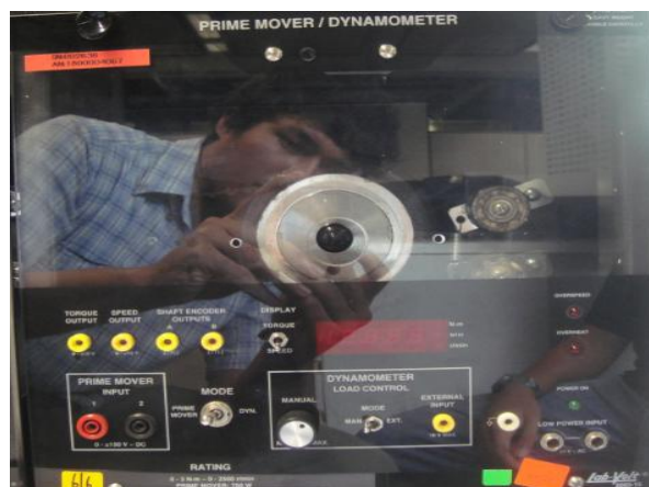
Figure 18. Lab Scaled Prime Mover/Dynamometer
