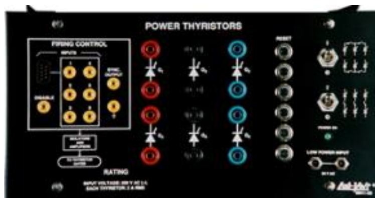
Figure 24. Lab scaled power thyristors
