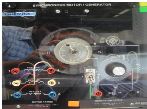
Figure 17. Lab scaled three phase synchronous generator
