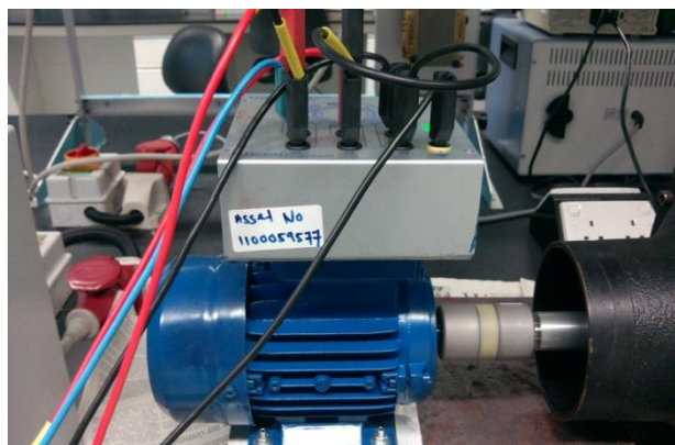
Figure 10: The squirrel cage 0.23kW motor used for experiment
