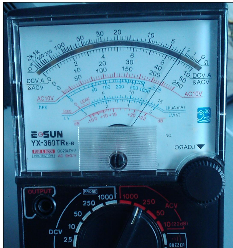
Figure 29: Analog multimeter showing steady-state value of loaded system voltage (220V), 250-V, Red scale
