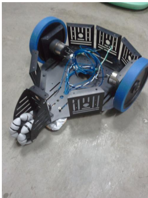
Figure 29: The Isolation Ward Dispenser Robot Base with two 7.2V DC Motors attached to the Wheels
