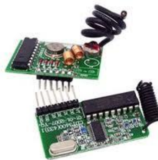
Figure 14: Transmitter and Receiver as Emergency Buttons
