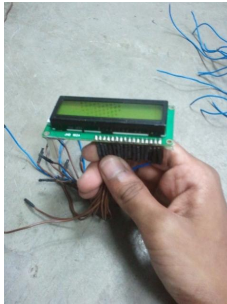
Figure 33: The 2x16 LCD Display for Patient Name Display
