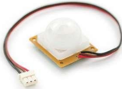
Figure 20: PIR Sensor Module
