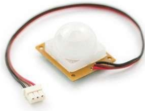
Figure 9: PIR Sensor Module
