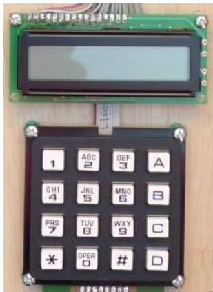
Figure 12: Keypad and LCD Integration
