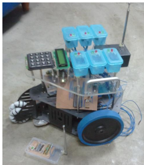
Figure 27: The Isolation Ward Dispenser Platform
