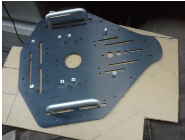
Figure 30: Acrylic Forming the Upper Level of the Isolation Ward Dispenser Robot
