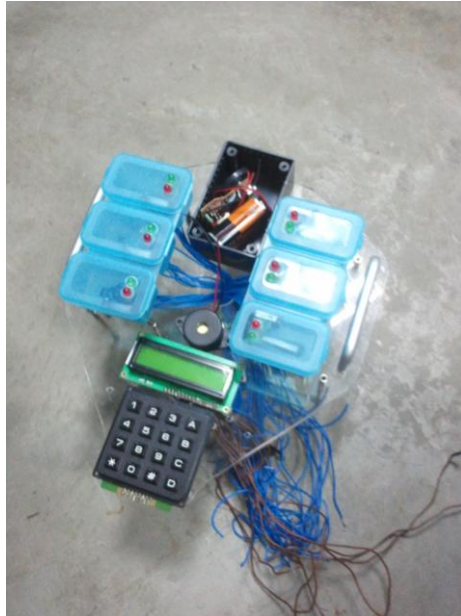
Figure 39: After Placing the Components Onto the Upper Level of the Isolation Ward Dispenser Robot
