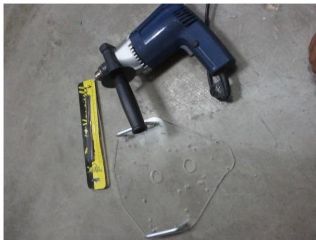
Figure 31: Acrylic Forming Upper Level of the Isolation Ward Dispenser Robot After Cutting and Drilling Process
