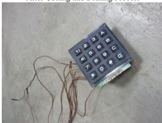
Figure 32: The 4x4 Keypad as the Password Input Device
