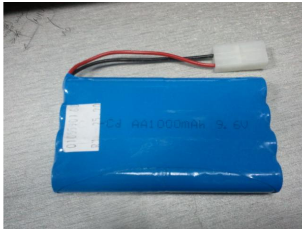
Figure 41: The 9.6V Ni Cd Rechargeable Battery Pack as the Power Supply
