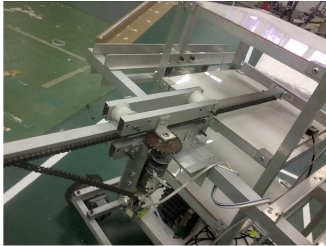
Figure [34]: Chain mechanism pushing the parcel/letter out of the compartment onto the receiving end
