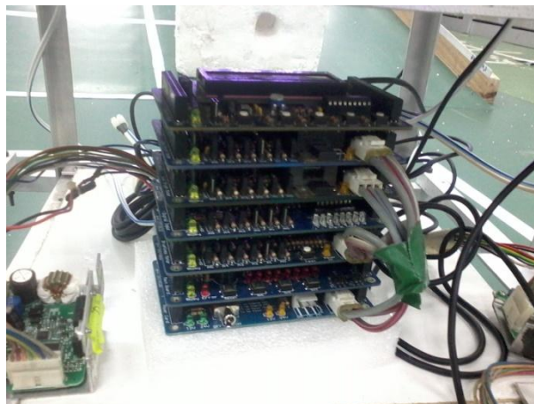
Figure [37]: IFC boards for the sensors and motors used for the robot
