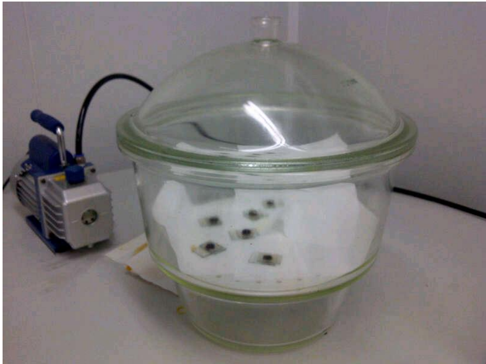
Figure 12: electrolyte filling process
