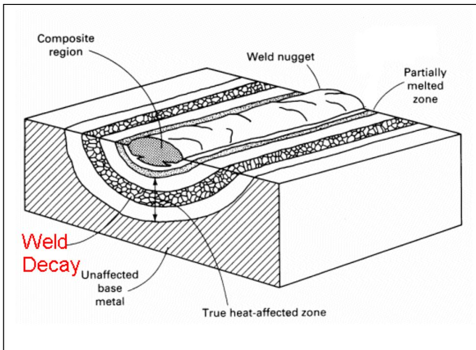
Figure 2.2: Schematic Diagram of Heat Affected Zone (HAZ)
