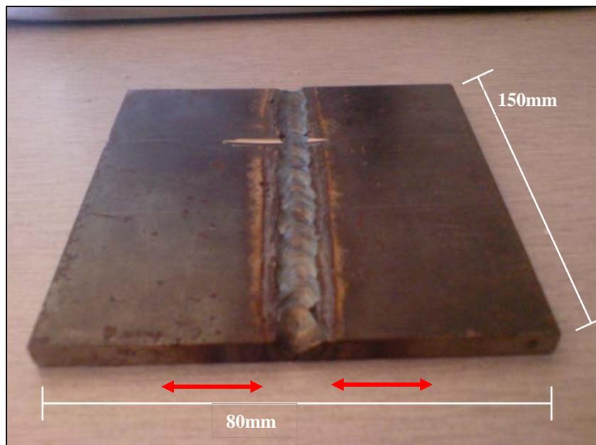
Figure 4.1: Area which Exposed to High Temperature.
