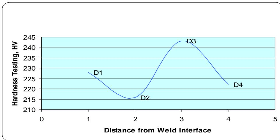
Figure 4.10: Hardness testing profile against distance from weld interface for 9mm thickness
