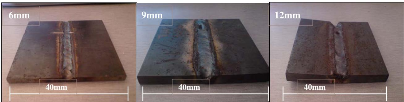
Figure 3.7: Finished Welding Material for Thickness of 6mm, 9mm and 12mm.
