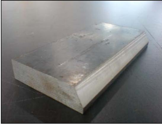
Figure 3.3: Finish Bevel Material
