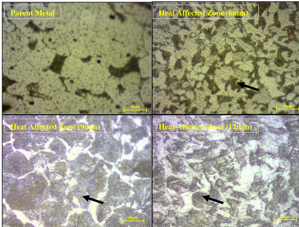
Figure 4.7: Comparison Microstructure between Parent Metal (100x) area and Heat Affected Zone (100x). Pearlite Microstructure layer (lamellar) can be seen clearly at arrow shown above.
