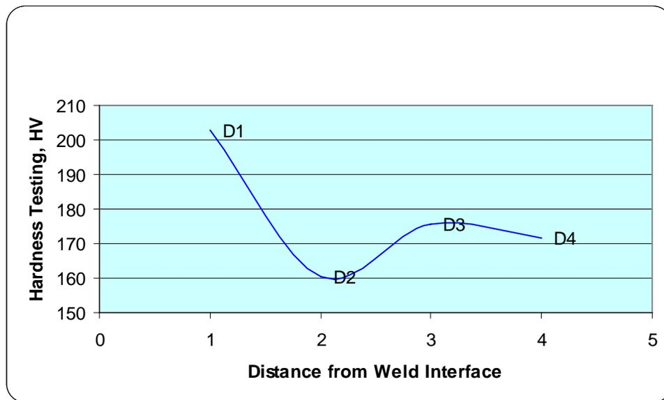
Figure 4.9: Hardness testing profile against distance from weld interface for 6mm thickness
