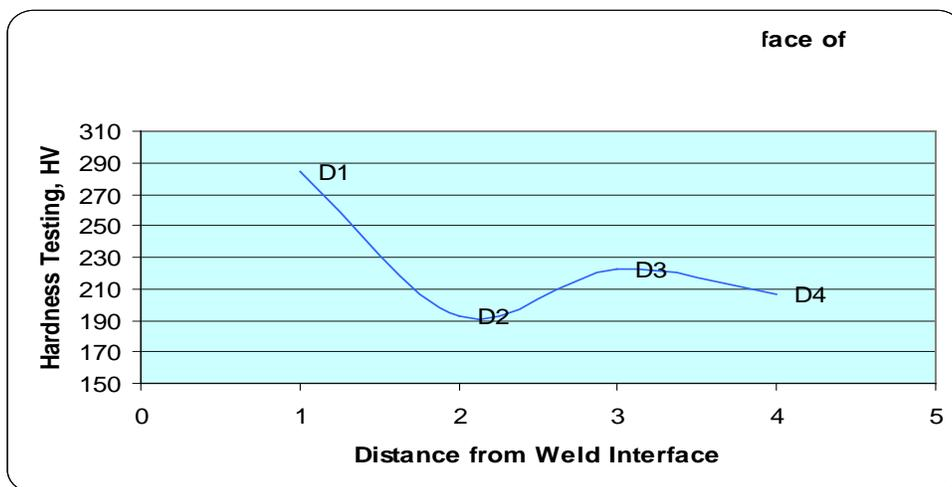
Figure 4.11: Hardness testing profile against distance from weld interface for 12mm thickness.
