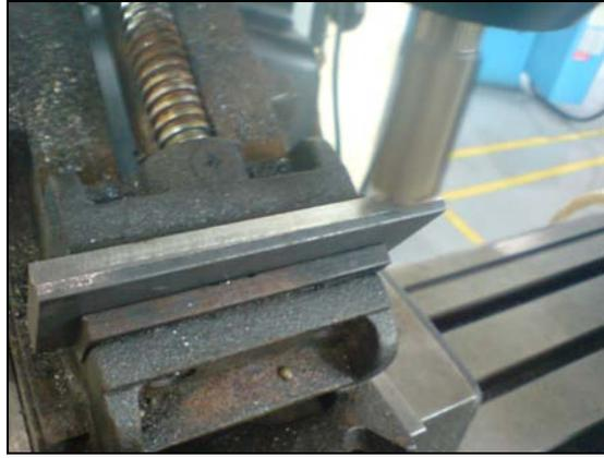
Figure 3.4: Milling Process for Beveling.
