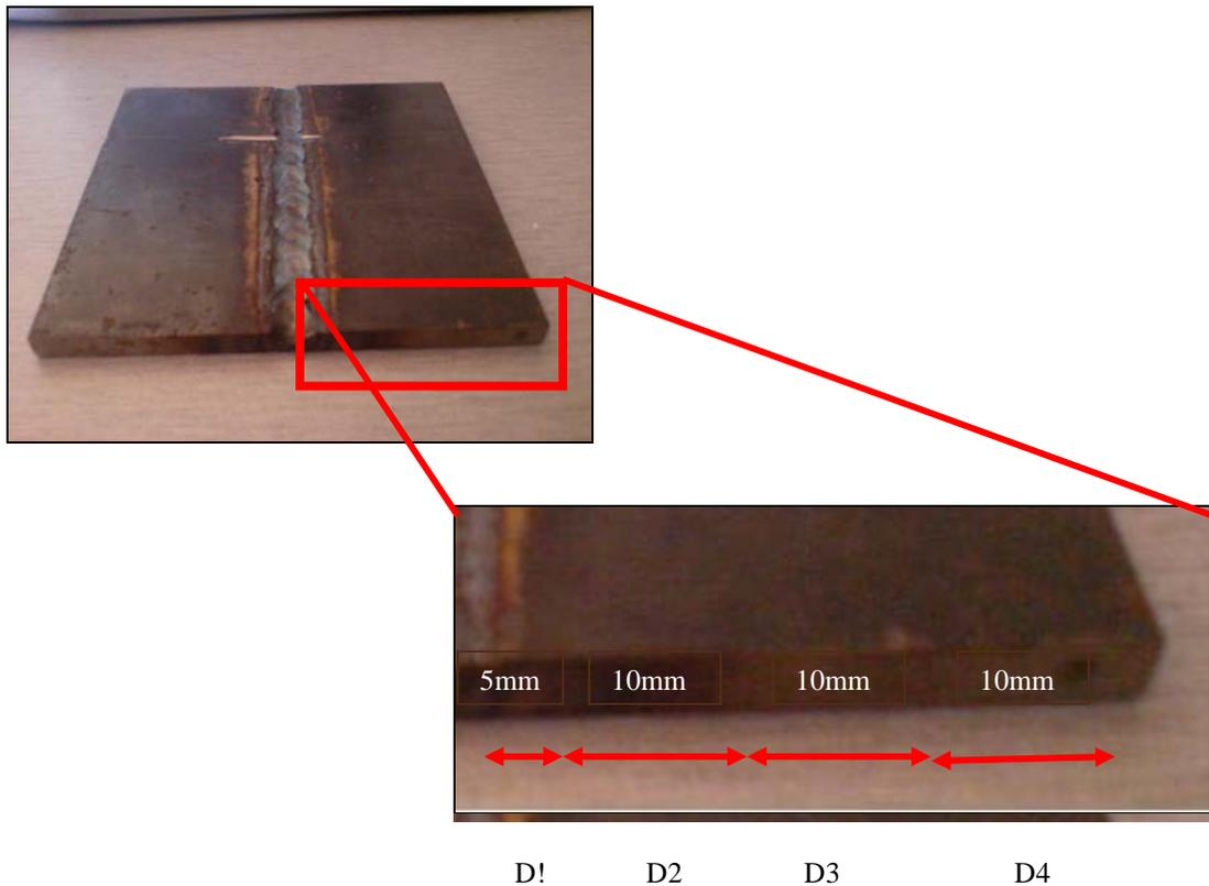
Figure 4.8: Testing areas adjacent to the fusion zone.
