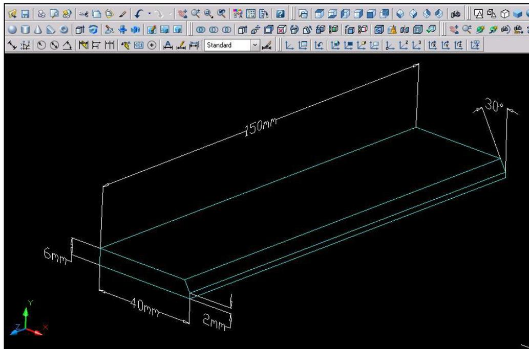
Figure 3.2: Bevel Configuration
