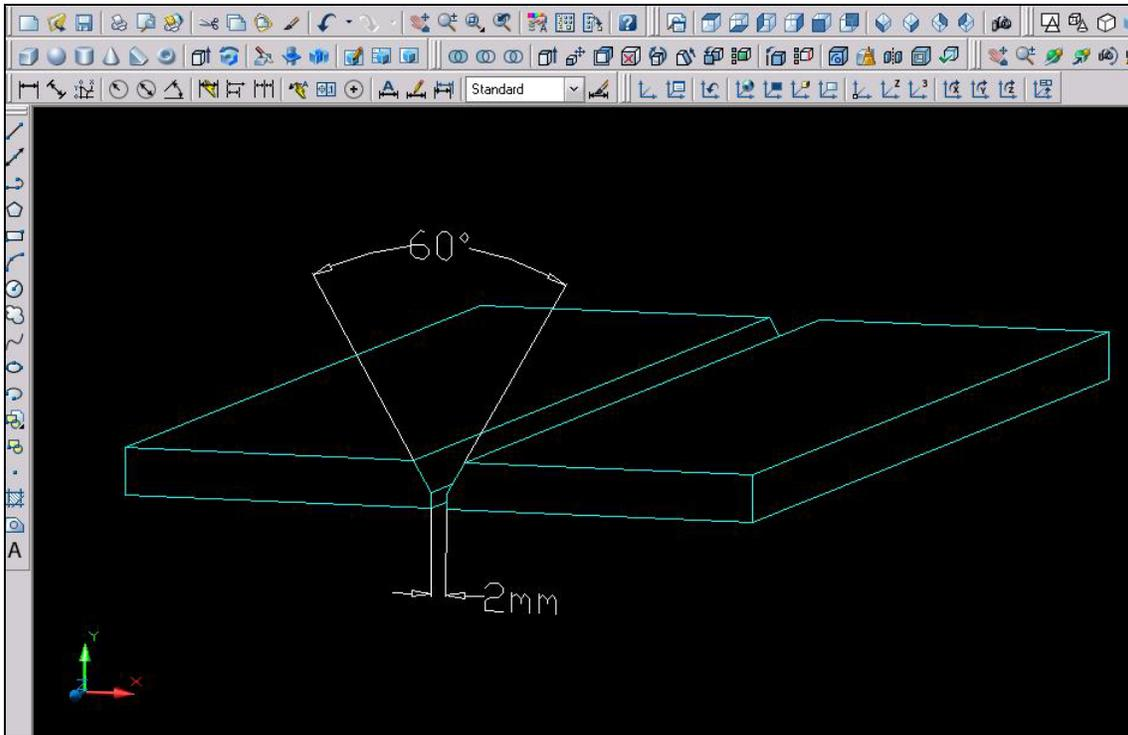
Figure 3.5: V Joint Arrangement for welding
