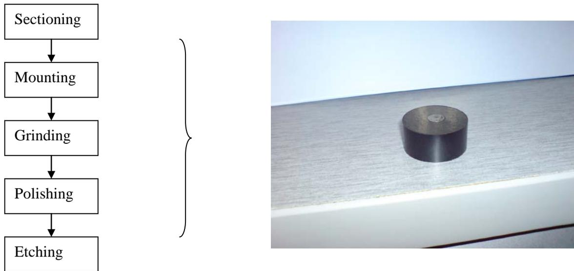
Figure 3.8: Metallographic sample preparation and example of specimen.
