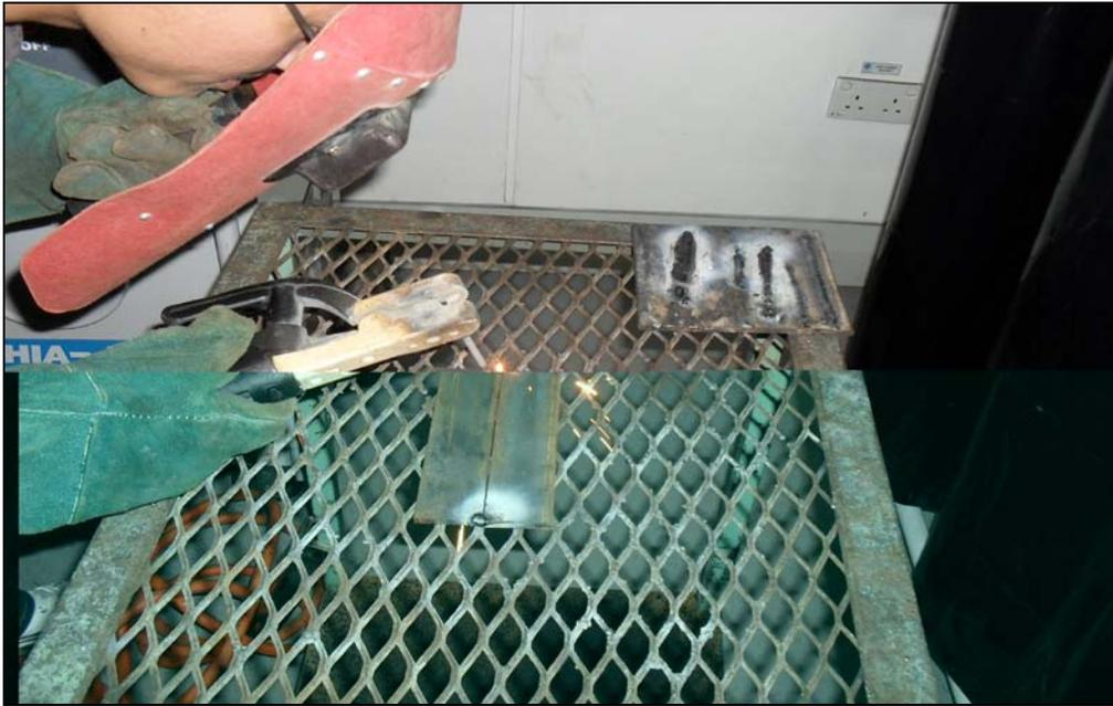
Figure 3.6: Welding Process – Shielded Metal Arc Welding
