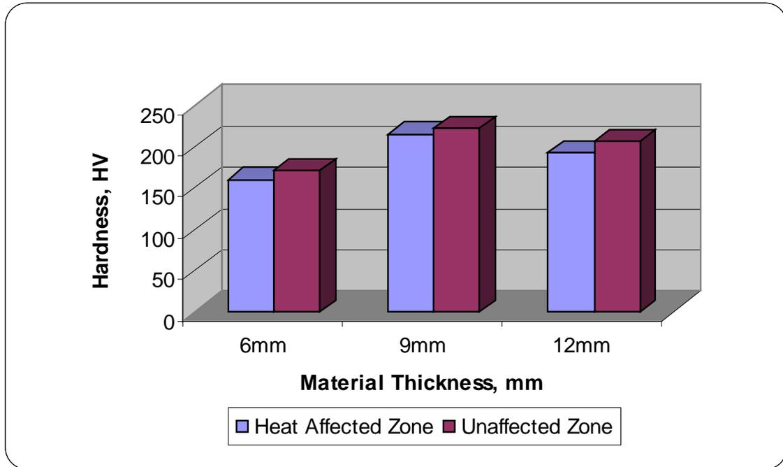
Figure 4.12: Comparison between heat affected zone and unaffected zone for various thickness.
