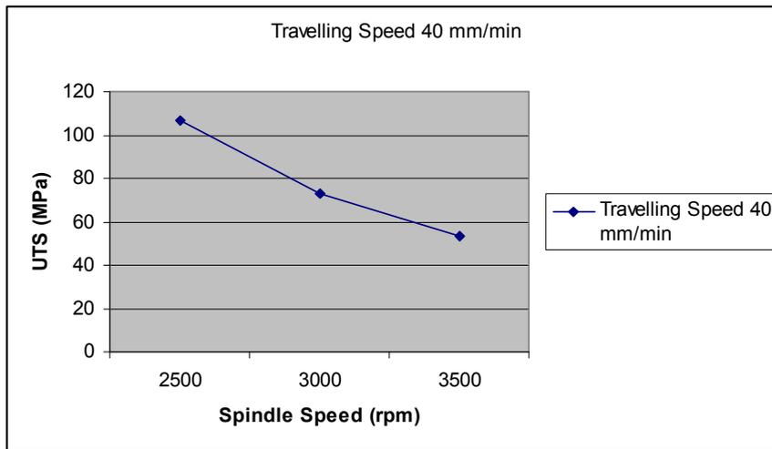
**Figure 23: UTS vs Spindle Speed graph with fixed Travelling Speed at 40 mm/min**
