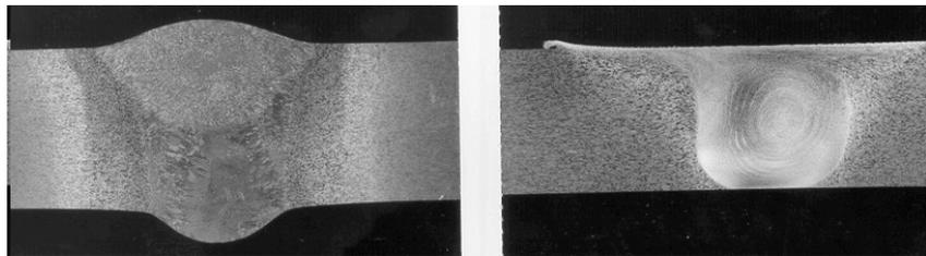
**Figure 2 : Weld nugget cross section [2]**
