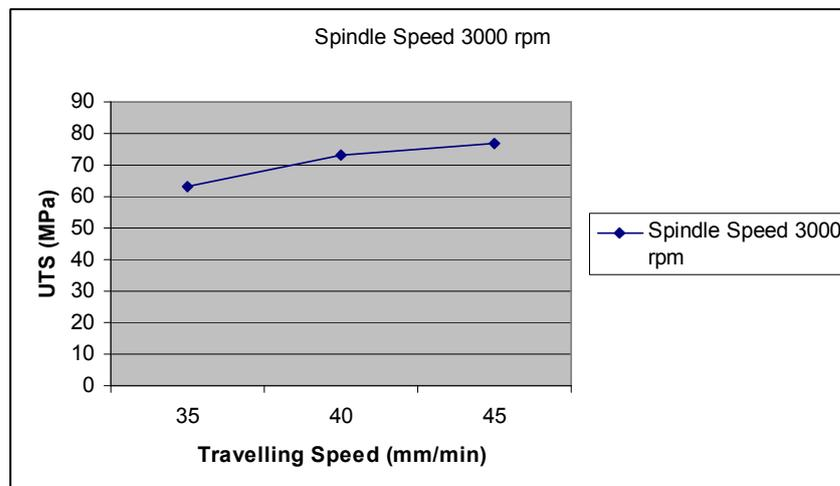
**Figure 22: UTS vs Travelling Speed graph with fixed Spindle Speed at 3000 rpm**
