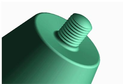
Figure 3 : Typical Weld Tool Profile
