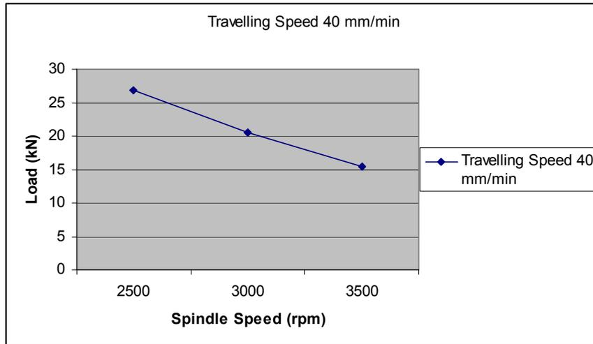
**Figure 21: Load vs Spindle Speed graph with fixed Travelling Speed at 40 mm/min**
