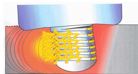
Figure 4 : Cross section of tool during stir action takes place <sup>[7]</sup>
