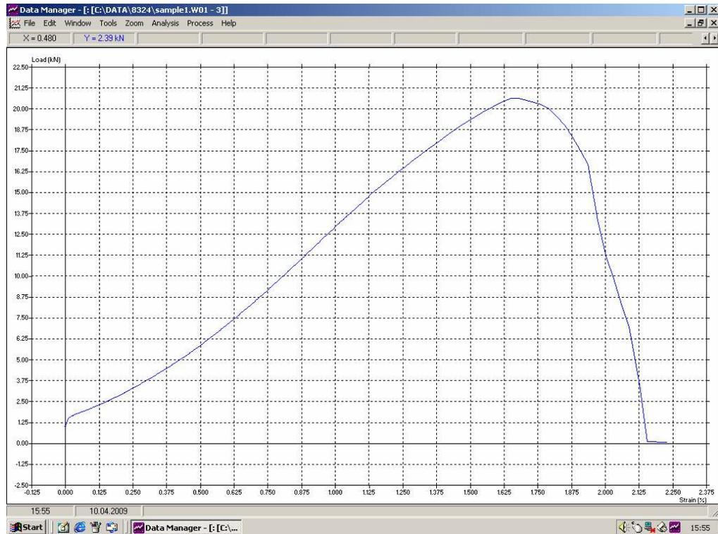
**Figure 16: Experiment 5 - Test Result (Load vs Strain)**
