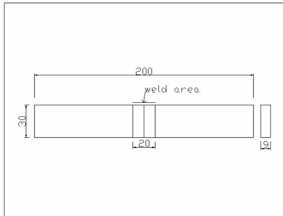
**Figure 7: Testing Dimension (in mm)**
