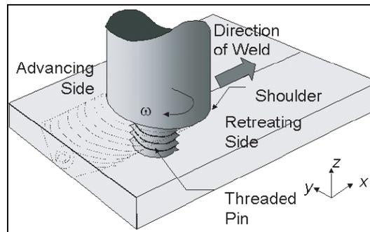
Figure 1 : Schematic diagram of FSW process<sup>[1]</sup>
