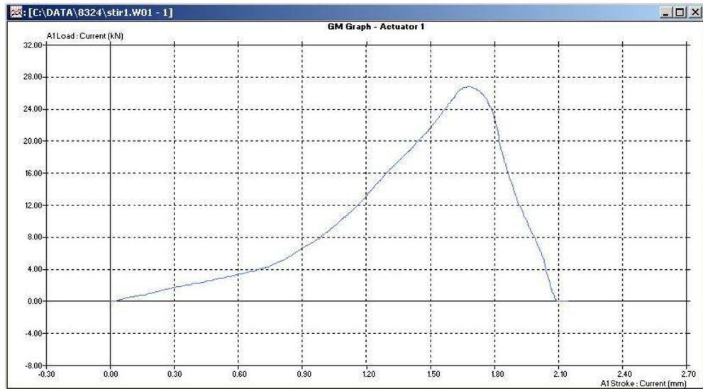
**Figure 19: Experiment 8 - Test Result (Load vs Strain)**
