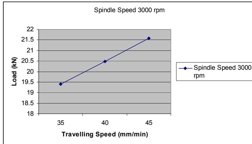
**Figure 20: Load vs Travelling Speed graph with fixed Spindle Speed at 3000 rpm**
