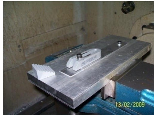
Figure 4.4: base plate clamping with jig
