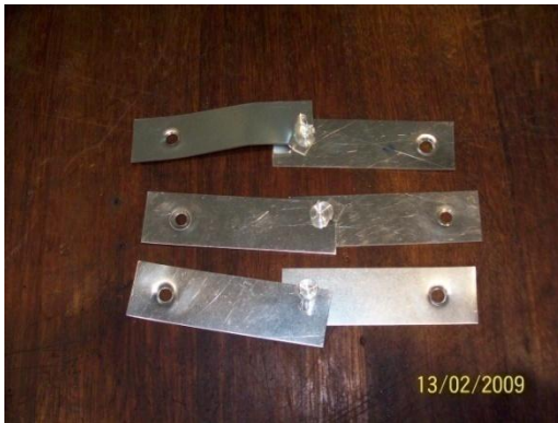
Figure 4.3: First try FSSW technique
