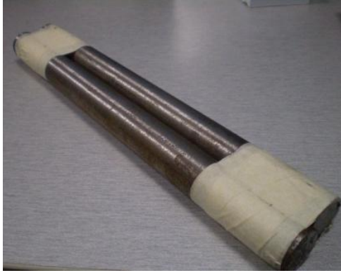
Figure 4.1: H13 hot work steel
