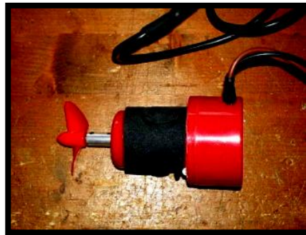
Figure 24: A Bilge Pump Thruster [11]
