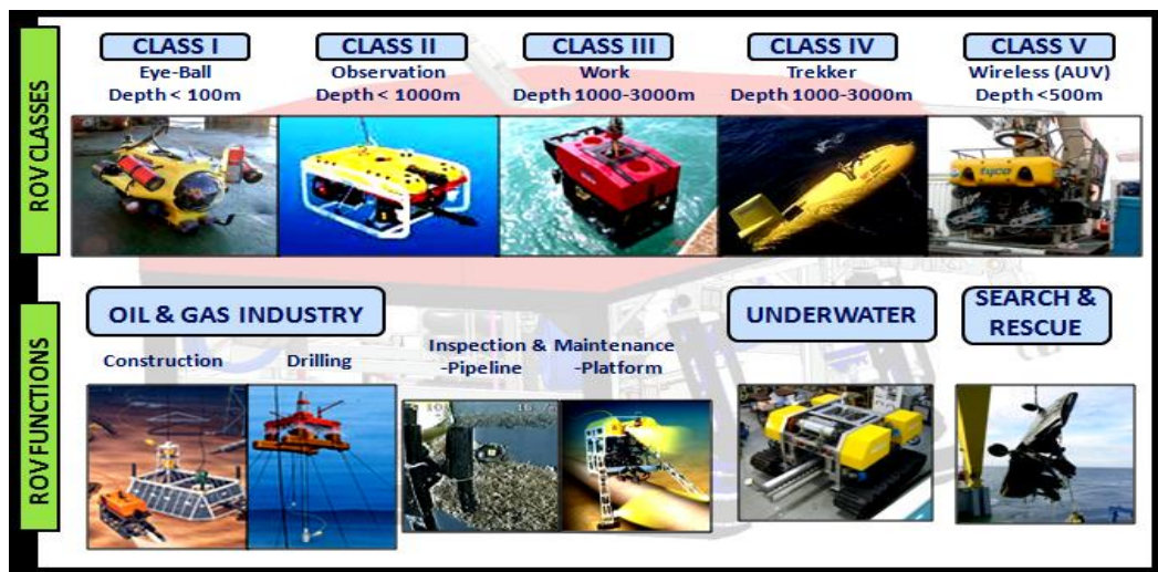
Figure 9: Remotely operated vehicle classes and functions [11]
