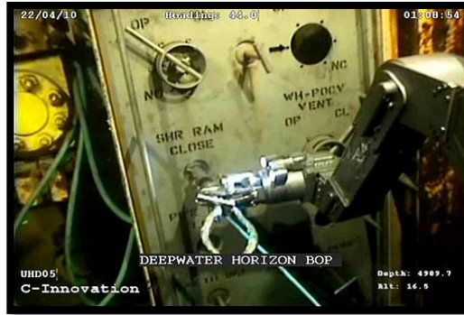
Figure2: Picture taken by the ROV while fixing the Blow Out Pressure that fails to react when the Leakage occurs at Deepwater Horizon Oil Rig [3]
