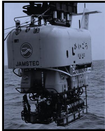
Figure 5: Kaiko – the world’s deepest diving ROV with 10909 m depth built by Japan [5]
