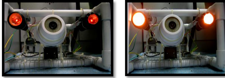
Figures 20: Light Dimmer Circuit Testing [11]
