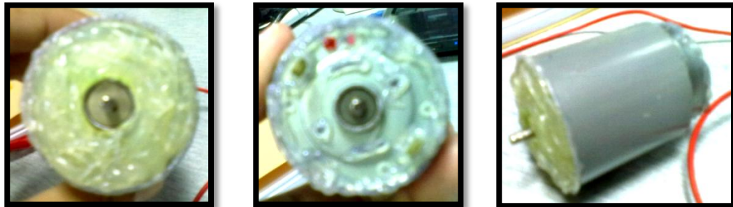
Figure 25: Waterproofing Process of the 12V DC Motor
