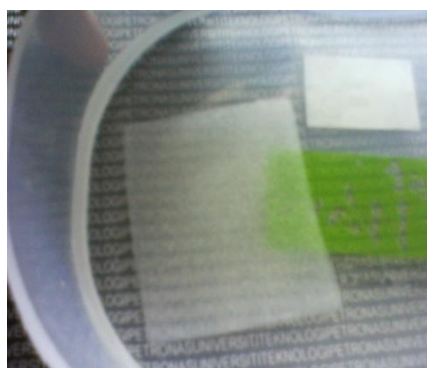
Figure 13: Sample condition after 5 days (10% mcc)
