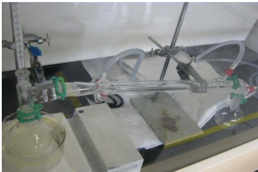
Figure 3.2: Experiment Set-Up for purification of pyridine
