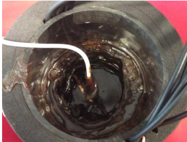
Figure 9 : Upper view of ECT that contains crude oil
