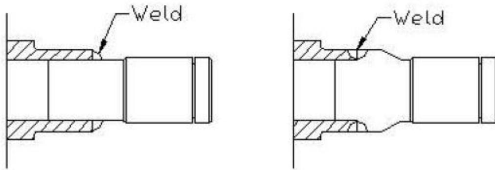
Figure 10 : Stub end weld design
