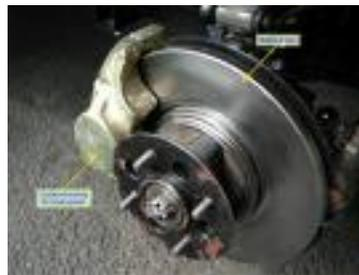
Figure 5: Disc Brake
