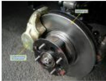
Figure 5: Disc Brake
