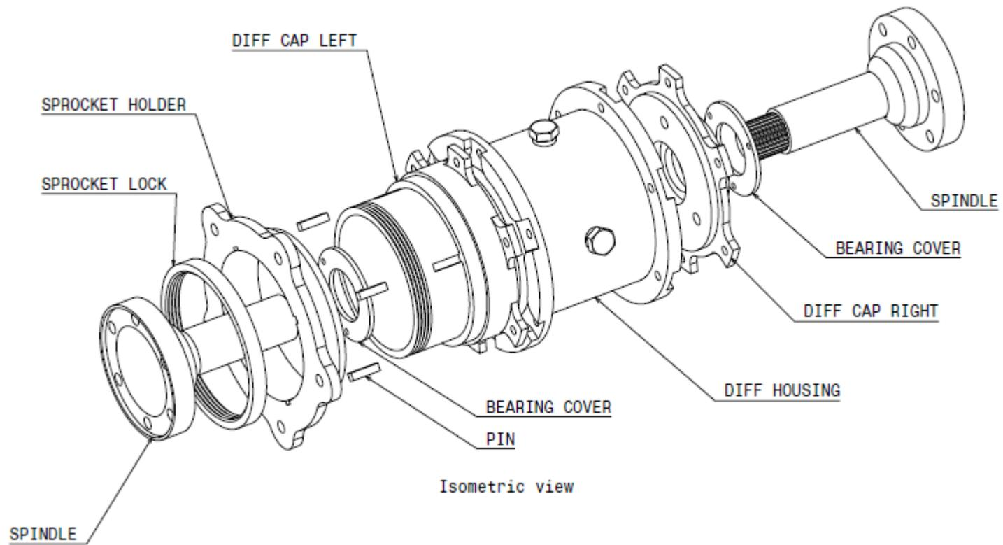
Figure 8 : 3 Dimension drawing of drive train
