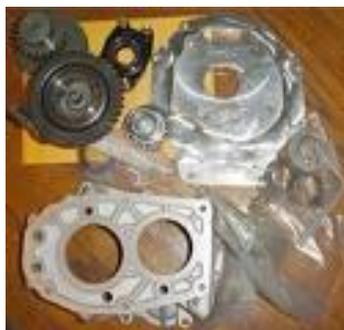
Figure 1 : Gear Reduction Box
