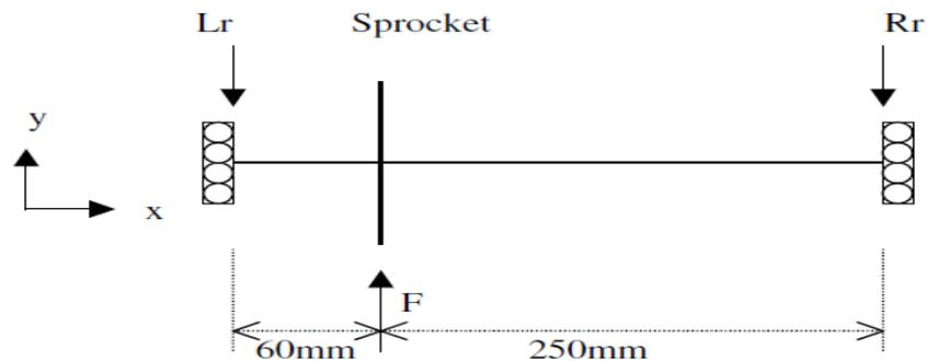
Figure 11: Free Body Diagram of Centre Shaft
