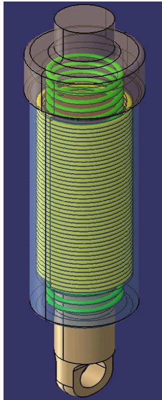
Figure 4.2.2: Assembled isometric view of the regenerative system
