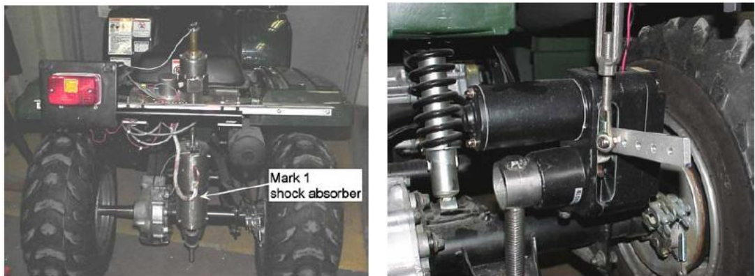
Figure 2.3.1: Mark 1 (left) and Mark 2 (right) shock absorber mounted on test vehicle
