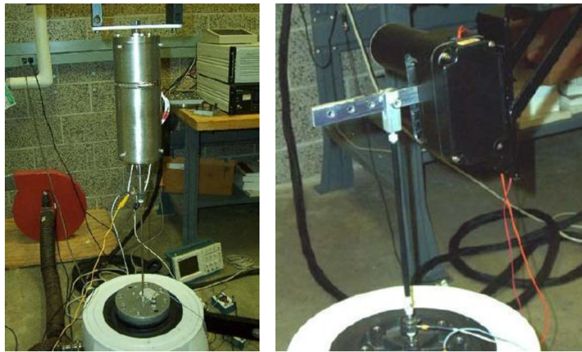
Figure 2.3.2: Mark 1 shock tested on electrodynamic shaker
