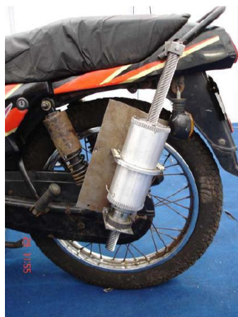
Figure 2.3.5: Prototype of the RSA mounted on a bike
