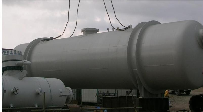
Figure 1: Horizontal Separator
