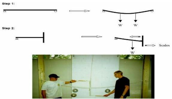
**Figure 3a**: Two students demonstrate moment in Lab. The "beam" is made out of PVC pipe. There are actually two PVC beams: one behind, to which a moment is being imparted by two hanging weights, and one in front, which is cut in half so that students can measure the amount of force required to duplicate the curve of the pipe behind it.
