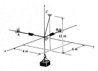
Q3. The pole for a power line is subjected to the two cable forces of 6 kN, each force lying in a plane parallel to the x-y plane. If the tension in the guy wire AB is 8 kN, determine the x, y, z, components of reaction at the fixed base of the pole, O due to these three forces.
