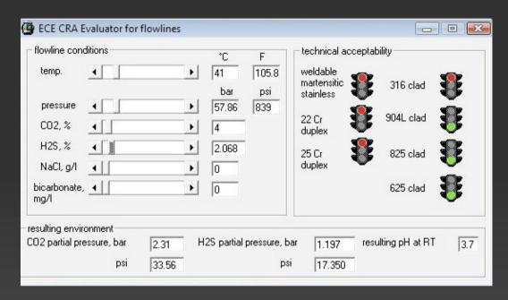
Even at low temperature (around 40°C), one by one material starts to fail its technical acceptability in the case of  $H_2S$  presence in  $CO_2$  environment.
