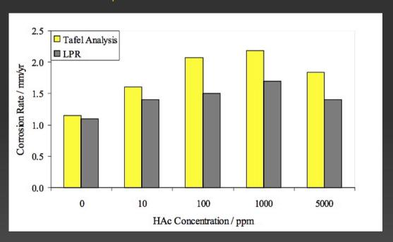
CR is not significantly affected by HAc at room temperature but at high temperature environment.
