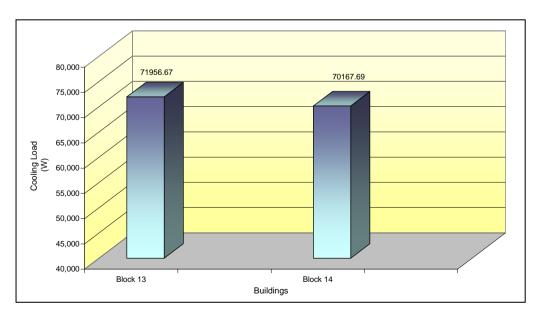
Figure 4.8 : Total cooling load for each buildings in Zone 4
