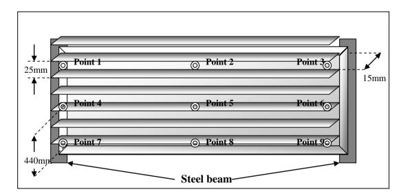
Figure 4.14 : Schematic diagram of the experiment
