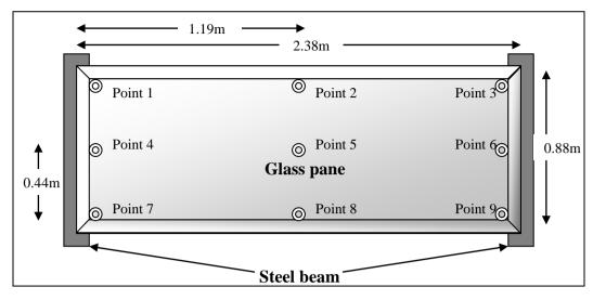
Figure 4.11: Schematic diagram of the glass pane
