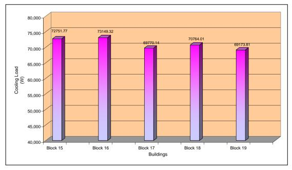
Figure 4.6 : Total cooling load for each buildings in Zone 2
