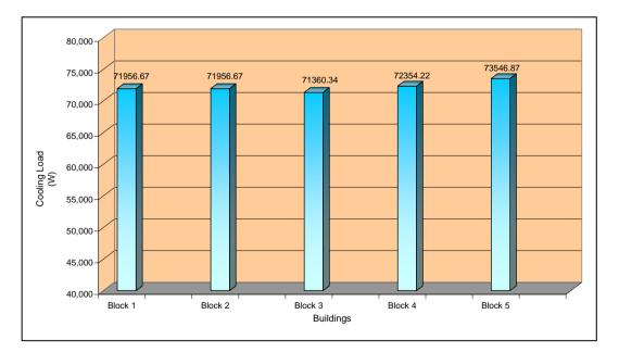
Figure 4.7 : Total cooling load for each buildings in Zone 3
