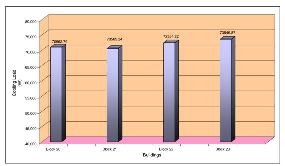
Figure 4.5 : Total cooling load for each buildings in Zone 1
