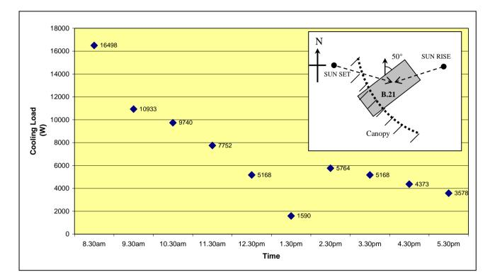
Figure 4.4 : Cooling Load Pattern According to Time on 4<sup>th</sup> March 2009. The inset pictures shows the diagram of Block 21
