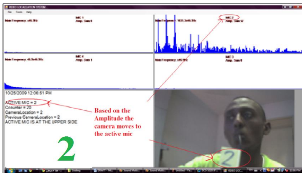
Figure 19: Localization results shown for MIC 2.
