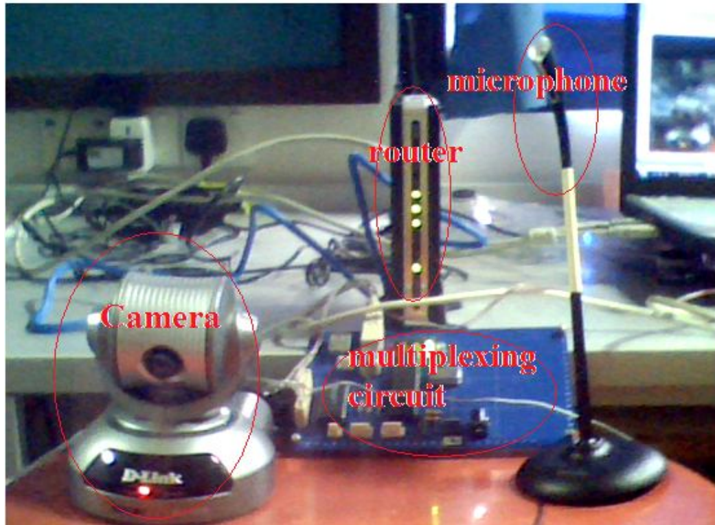
Figure 23: System components that been used in this project.
