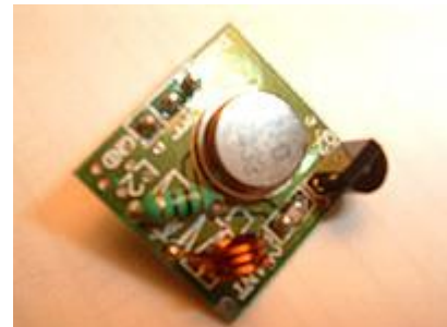
Figure 11: RF transmitter module CS901
