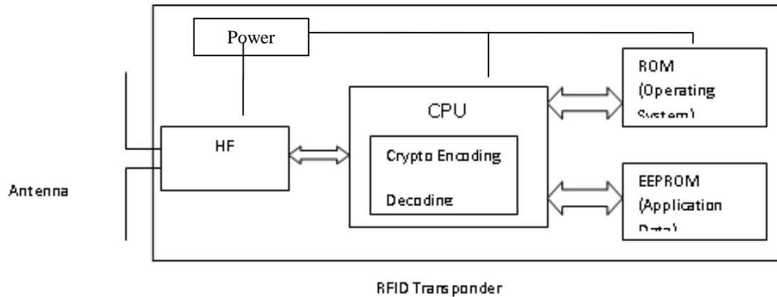
**Figure 4: Block Diagram of Active RFID Tag**
