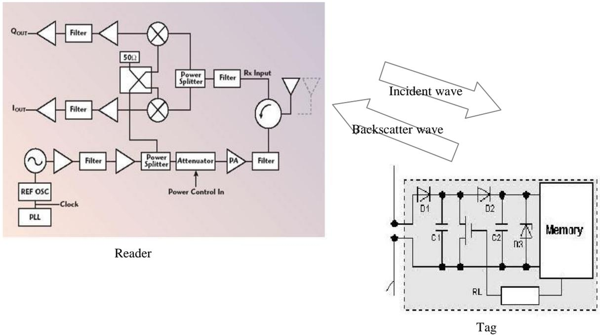
**Figure 2 : Backscatter modulation circuitry**
