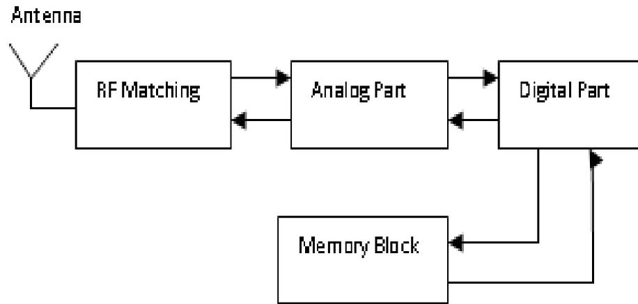
**Figure 3: Block Diagram of Passive RFID Tag**
