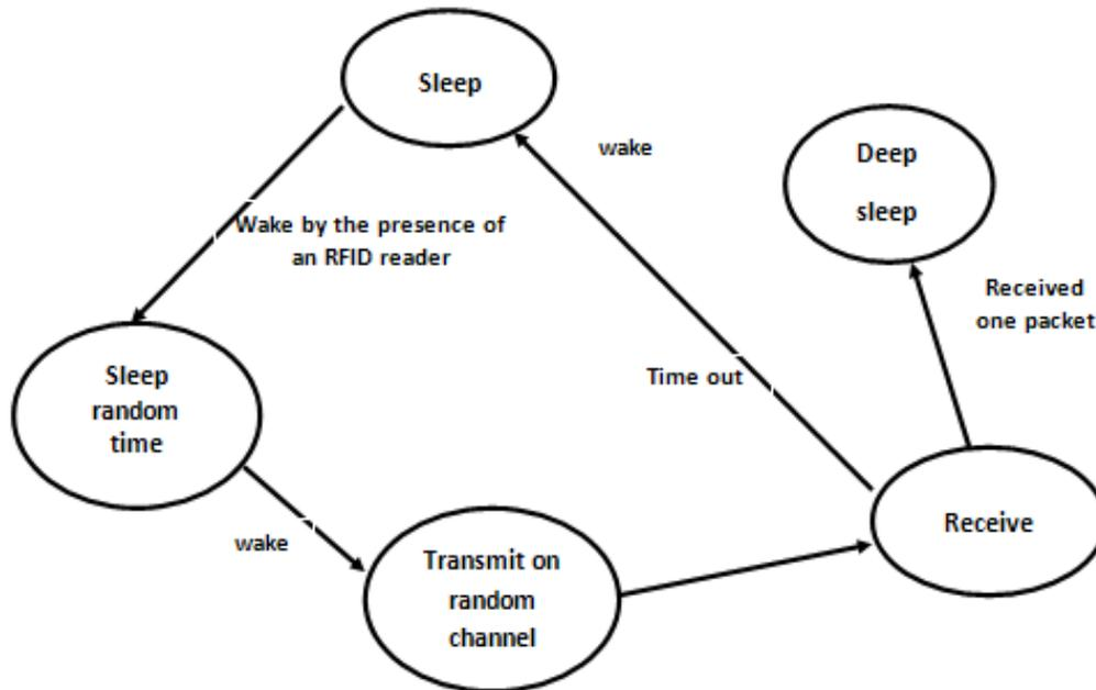
**Figure 5: State diagram of a tag executing the optimal protocol**
