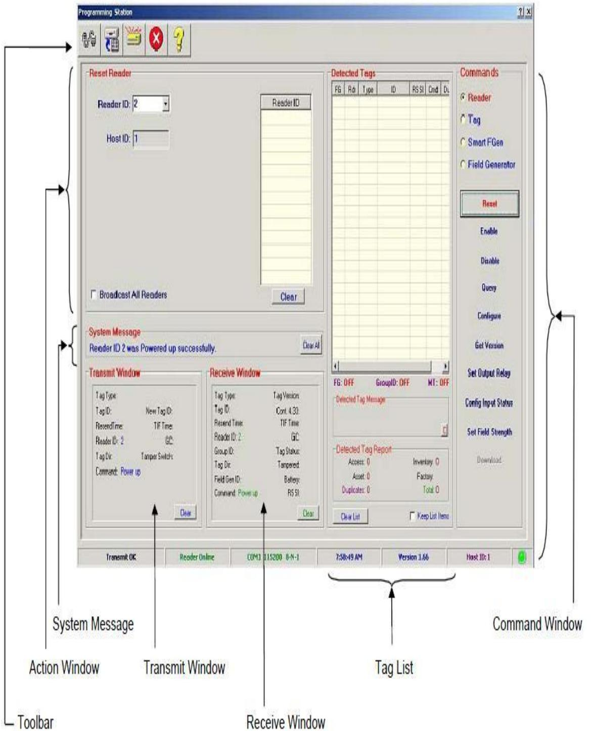
**Figure 8: Programming Station Main Screen**
