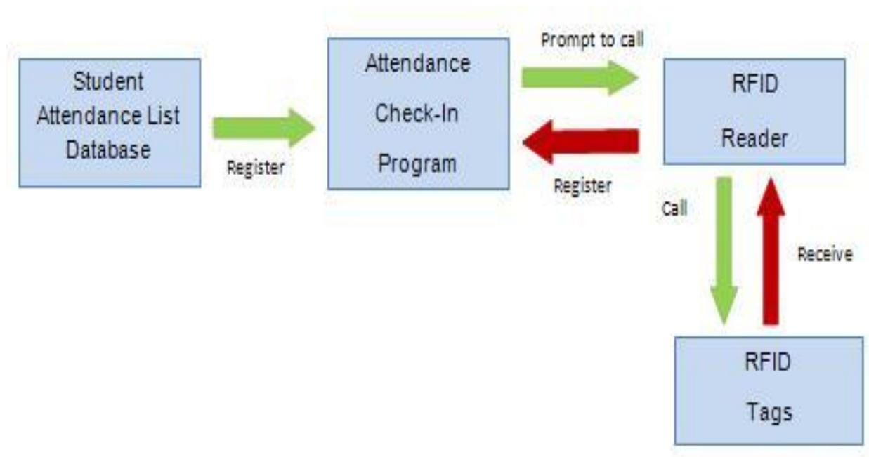
Figure 10: Software and Hardware Establishment
