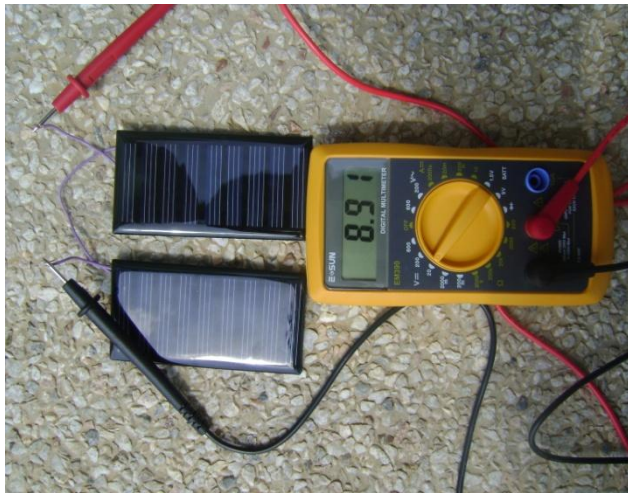
Figure 12: Testing solar panel using multimeter (cloudy day)
