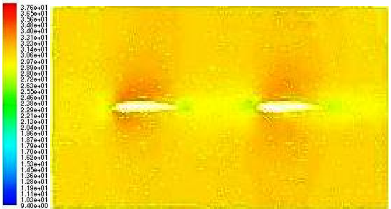
Figure 4.20: Velocity vectors for two airfoils separated at one chord length, 0.13 m at 0° AoA at 30 m/s
