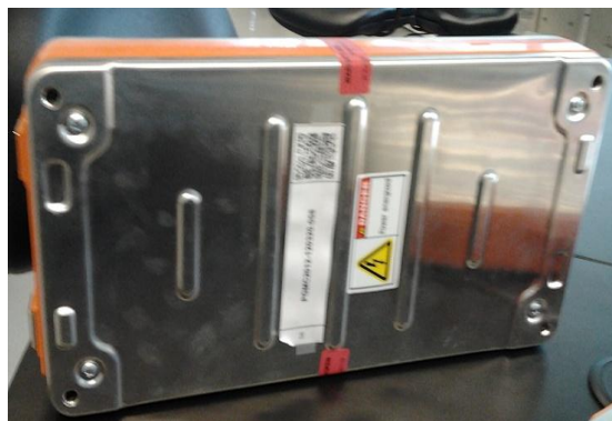
Figure 3.3: Side view of Lithium-ion Battery (1 Module)
