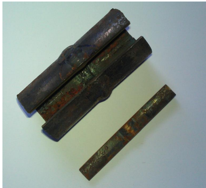
Figure 3.3: A longitudinal part (approximately 1cm in width) was cut from the shortened pipe for metallographic analysis
