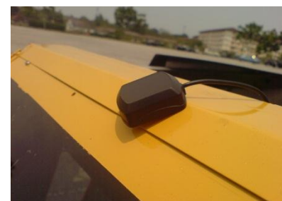
Figure 3.6: Receiver for data logger installed at the car
